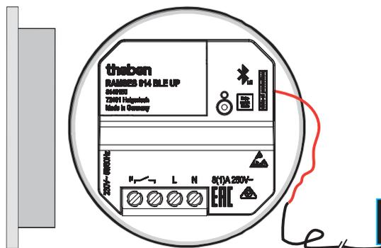
The two insulated ends of the plugged in sensor cable form the external input.
